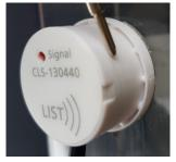
**Step 1/** Carefully remove the rear cover of the sensor using wither your fingers, or a fine (jeweller's) screwdriver.
