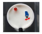
**Step 3/** Adjust the sensor sensitivity according to your requirements, in increments of 1/4 turn between tests
